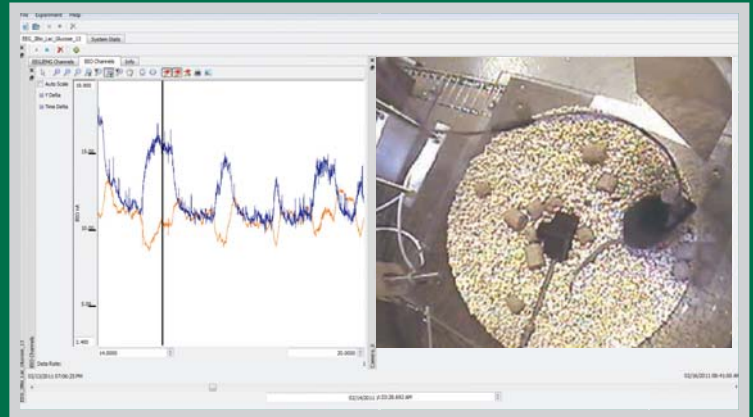
Biosensor traces for lactate and glucose are recorded simultaneously with full-color video.
