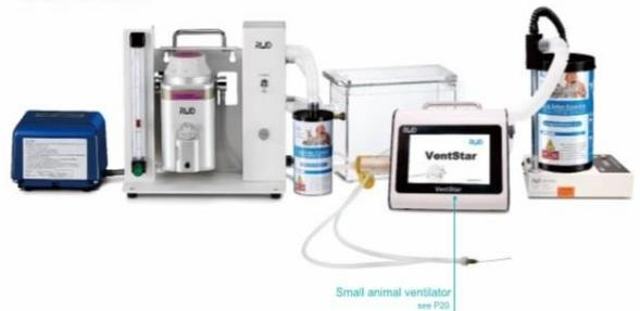
This program is the combination of anesthesia machine and ventilator. While keeping the animal under anesthesia, it provides a certain volume (tidal volume) of oxygen and respiratory rate to support the normal breathing of animals.
