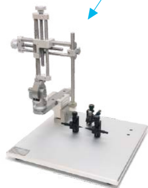
Portable Stereotaxic Instrument The height of the teeth bar and ear bar can be adjusted for easy adjustment of the cranial level.
