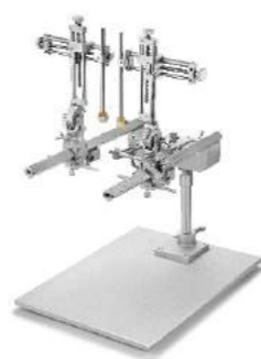
Large Animal Stereotaxic Instrument Used to stereotaxic experiments of cats, dogs, monkeys and other large animals.
