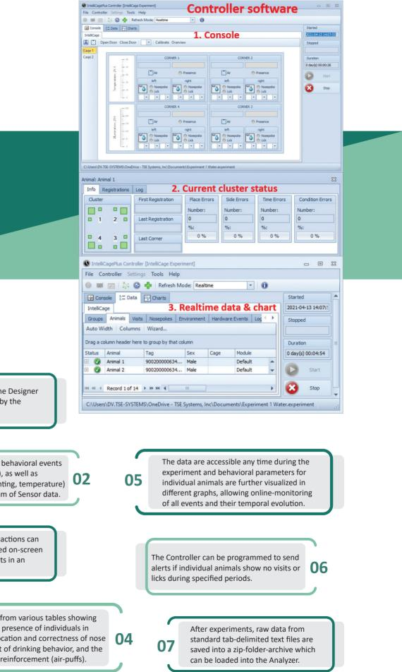
Experimental files from the Designer are loaded and executed by the Controller software
