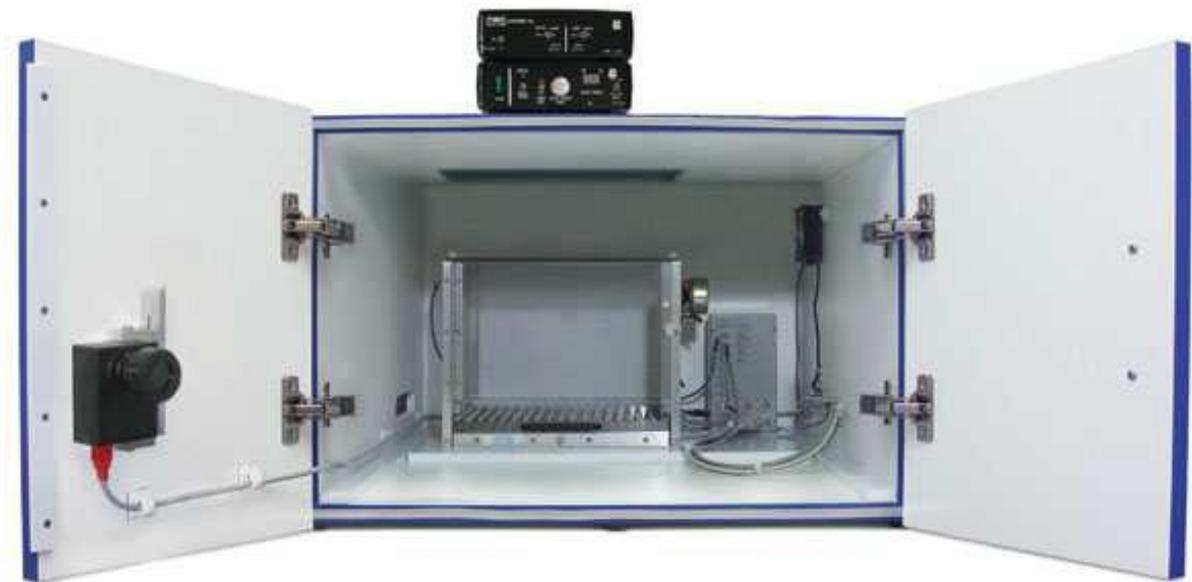
Eliminate the need for bright visible light by taking advantage of our new NIR-based imaging system. Bright visible lighting yields uniform illumination, which is essential for high quality, low-noise video recording of animal behavior. However, in some instances, this bright illumination may adversely impact animal behavior by serving as a contextual cue to the animal.
